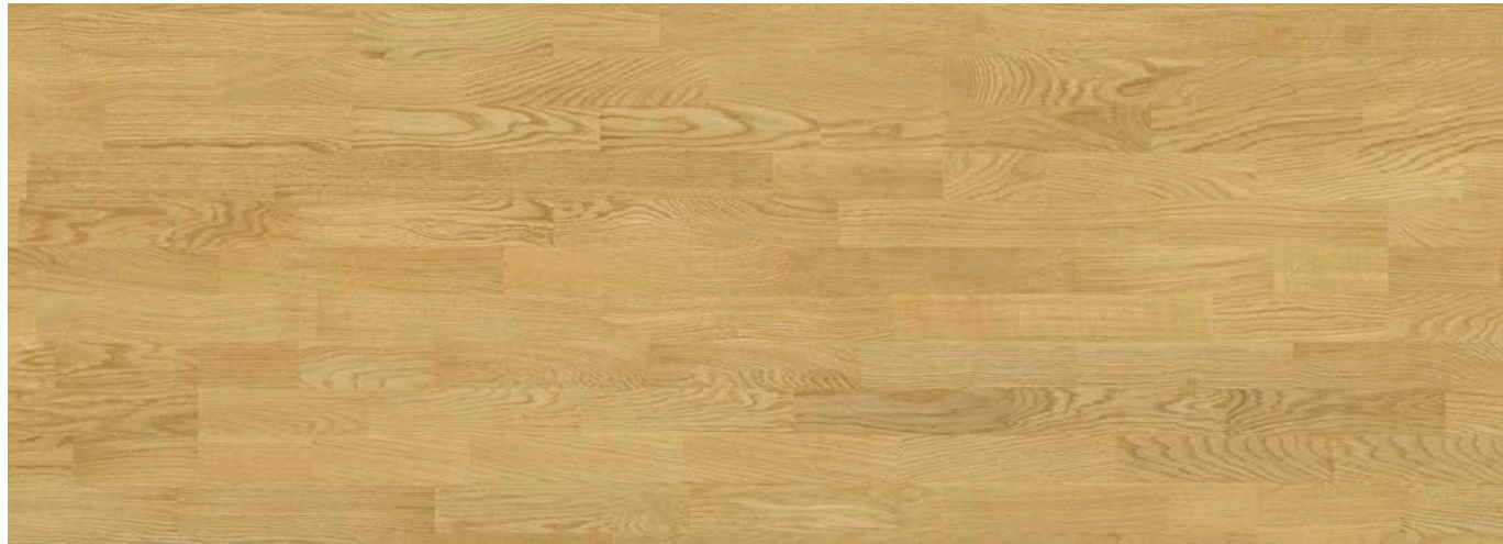
3 Strip Oak City Very light natural color variation. Sapwood not allowed, healthy knots diameter below 5 mm, no repaired knots
