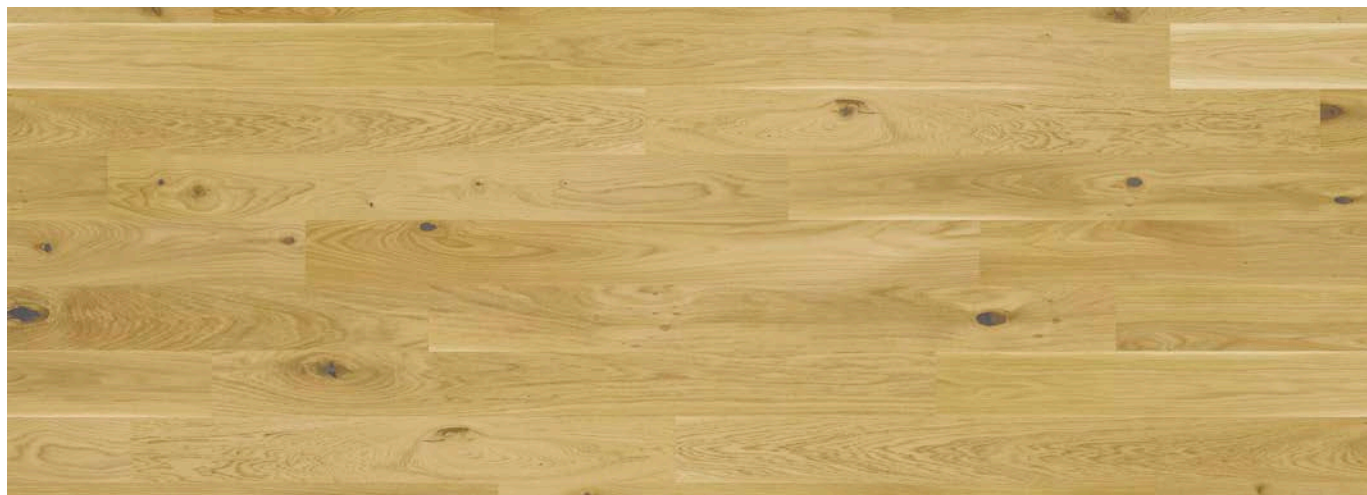
1 Strip Oak Ranch Higher color variation allowed. Occasional sapwood below 50 mm width, unlimited healthy knots and fallen out repaired knots diameter below 60 mm, filled crack < 150 mm
